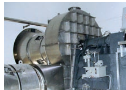
High-capacity fan for mechanical vapour recompression
