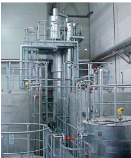
Two-effect evaporation plant for wood steaming waste water. Evaporation rate: 5,000 kg/h
