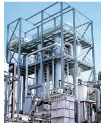
Two-effect forced circulation evaporation plant Evaporation rate: 12,000 kg/h
