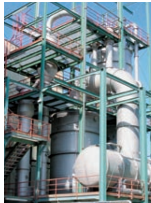
Falling film forced circulation evaporation plant, directly heated by turbine exhaust steam Evaporation rate: 31.000 kg/h
