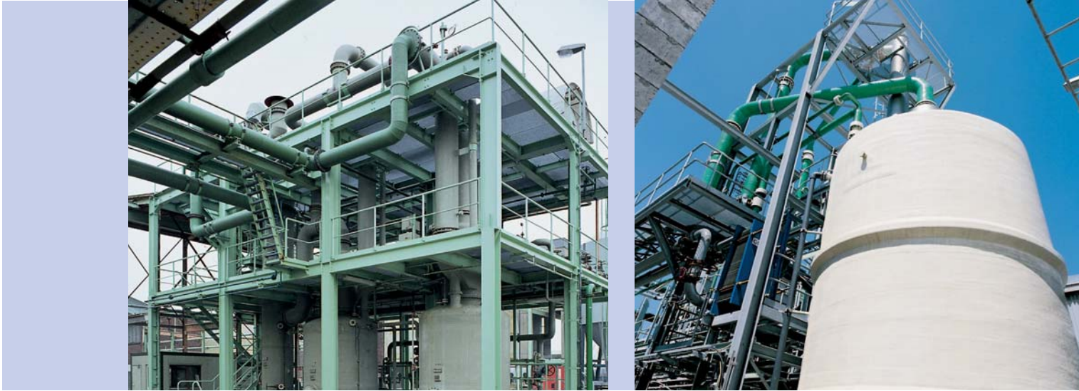
Lefthand fig.: Chloric gas absorption plant for cleaning exhaust air from chlor-alkali electrolysis and for the production of chlorine bleaching
