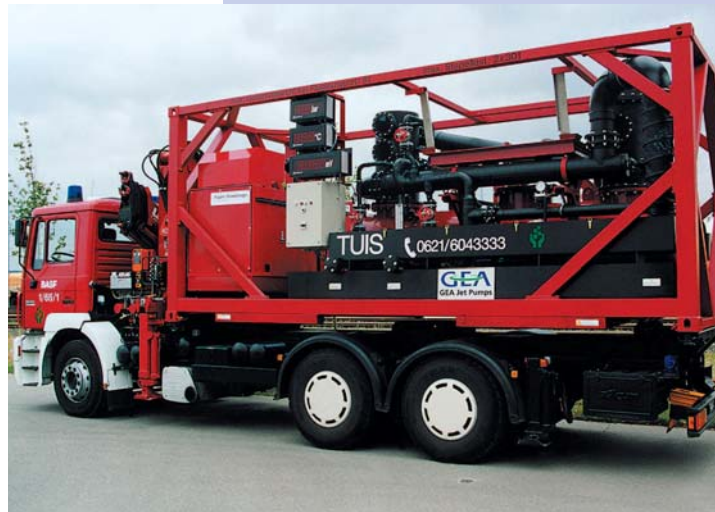
Mobile chlorine emergency unit in operation
