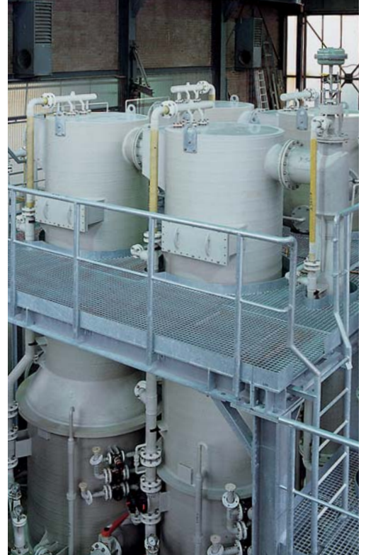
Jet scrubbing plant type II for acid and alkaline exhaust gases
