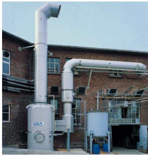
Single effect continuously adjustable Venturi scrubbing plant type U for washing out dusts suction flow: 30,000\ \text{m}^3/\text{h} pressure loss: 20 mbar
