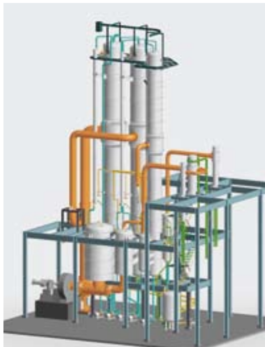
2-EFFECT FALLING FILM EVAPORATION PLANT with mechanical vapour recompression and single-effect falling film evaporator (finisher) with thermal vapour compressor and vacuum cooler for glucose DE 30 to DE 55 . Evaporation rate: 49,300 kg/h
