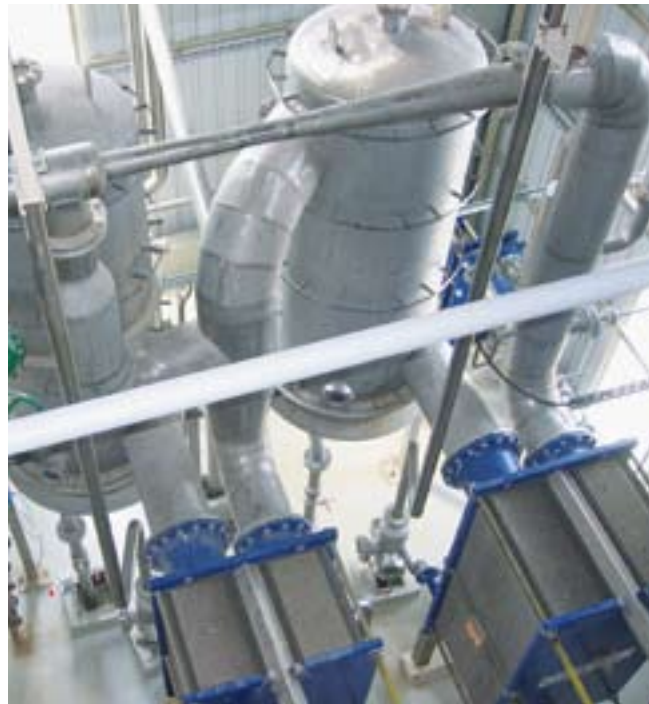
2-EFFECT PLATE EVAPORATION PLANT for sorbitol solution, heated via a thermal vapour recompressor. Evaporation rate: 4,300 kg/h
