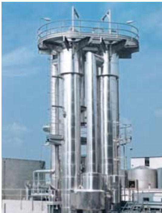
SINGLE-EFFECT FALLING FILM EVAPORATION PLANT with two parallel, multi-path calandria for two different starch hydrolysates, heated via a common mechanical vapour recompressor. Evaporation rate: 22,000 kg/h
